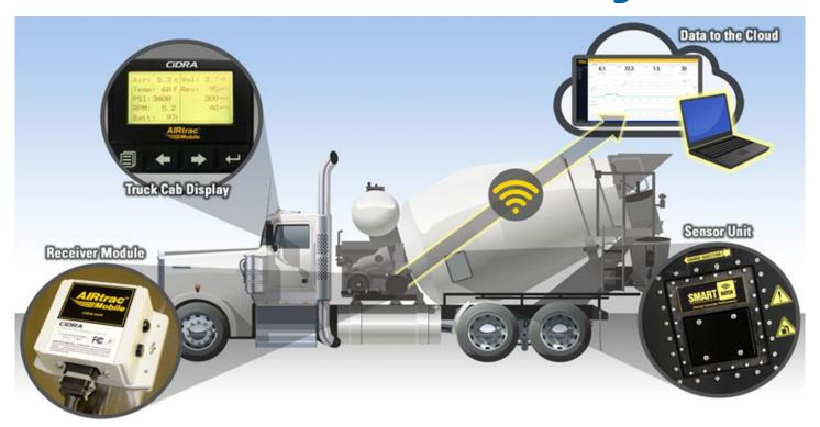
The SMARThatch system can easily be retrofitted to any style of concrete truck and is available for a flexible subscription fee that includes hardware at no additional cost. For concrete producers and truck operators, this solution translates into increased productivity, reduced waste, lower costs, and enhanced competitiveness.
