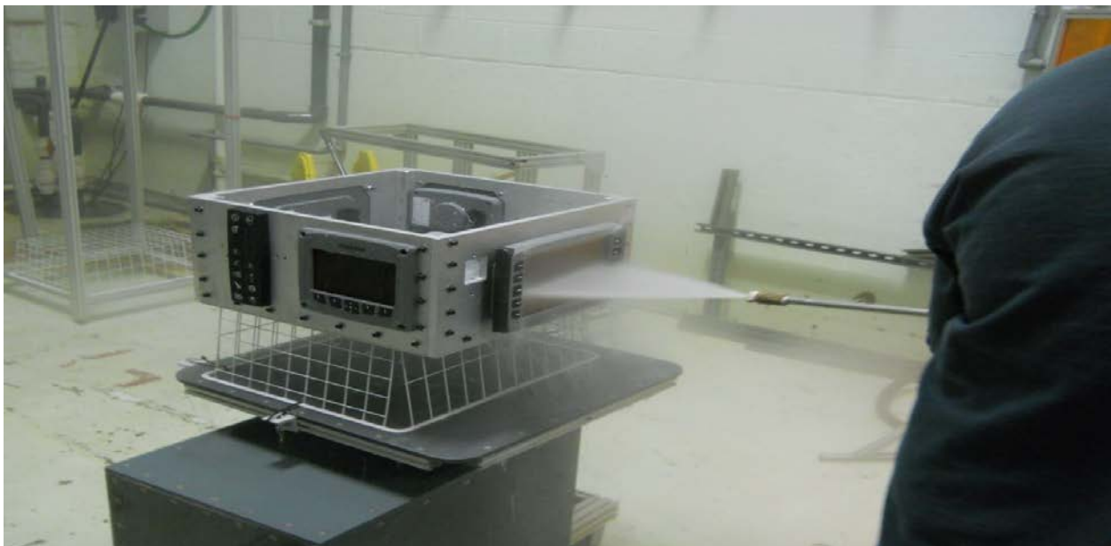
Washdown testing to confirm IP69K rating for ingress protection
